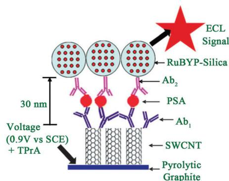
**Fig. 11** Scheme of representation of ECL-based SWCNT immunosensors after addition of PSA and  $[Ru-(bpy)_3]^{2+}$ -silica- $Ab_2$  nanoparticles. (Reprinted with permission from ref. 63. Copyright 2009 Royal Chemical Society.)
