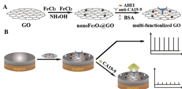
**Fig. 5** Schematic diagram for (A) the preparation of multi-functionalized graphene oxide, and (B) the fabrication and application protocol of the ECL immunosensor using multi-functionalized graphene oxide. (Reprinted with permission from ref. 47. Copyright 2015 Elsevier.)
