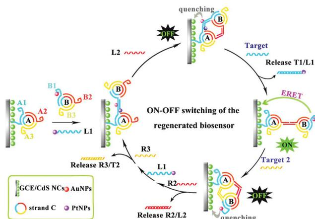
**Fig. 32** Operating principle of the dual miRNAs-fueled nanogear-based regenerated biosensor which realized the multiple ECL detection of miRNAs with a single luminophore. (Reprinted with permission from ref. 155. Copyright 2017 American Chemical Society.)
