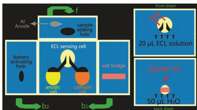
**Fig. 36** Schematic diagram of the working principle of a m-s-OECLD. f: Front sheet; b1: the sheet folded to the back first; b2: the back sheet. (Reprinted with permission from ref. 165. Copyright 2013 The Royal Society of Chemistry.)
