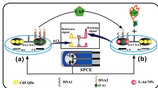
Fig. 26 Schematic illustration of the ratiometric ECL array for CAP quantification. (Reprinted with permission from ref. 89. Copyright 2015, Elsevier.)
