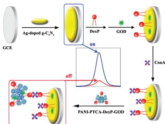
**Fig. 20** The illustration of the synthetic process of (A) Ag-g-C<sub>3</sub>N<sub>4</sub> and (B) PANI-PTCA-DexP-GOD, and (C) the preparation of the ECL biosensor. (Reprinted with permission from ref. 89. Copyright 2016, Elsevier.)
