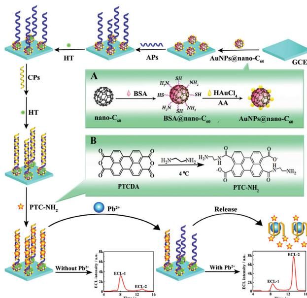
Fig. 22 Schematic illustration of the preparation process of the ratiometric aptasensor: inset of (A) and (B) display the preparation procedure of AuNPs@nano-C<sub>60</sub> and PTC-NH<sub>2</sub>. (Reprinted with permission from ref. 14. Copyright 2015, American Chemical Society.)
