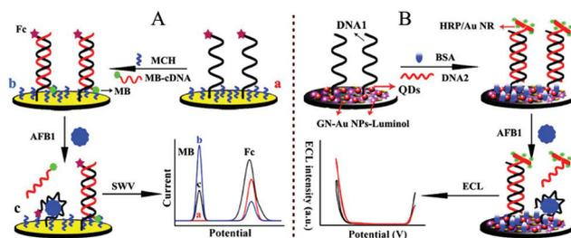
Fig. 25 Schematic illustration of the dual-signaling sensor for AFB1 assay with (A) electrochemistry and (B) electrochemiluminescence. (Reprinted with permission from ref. 121. Copyright 2017, American Chemical Society.)
