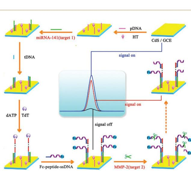
**Fig. 33** Fabrication of an ECL biosensing platform for the detection of multiple types of biomarkers on a single interface. (Reprinted with permission from ref. 157. Copyright 2017 American Chemical Society.)
