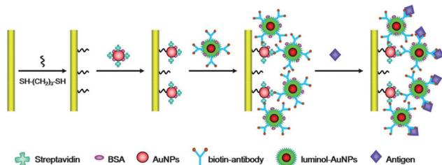
**Fig. 13** Schematic illustration of the fabrication processes of the label-free ECL immunosensor using luminol-AuNPs as antibody carriers and sensing platform. (Reprinted with permission from ref. 67. Copyright 2013 Royal Chemical Society.)
