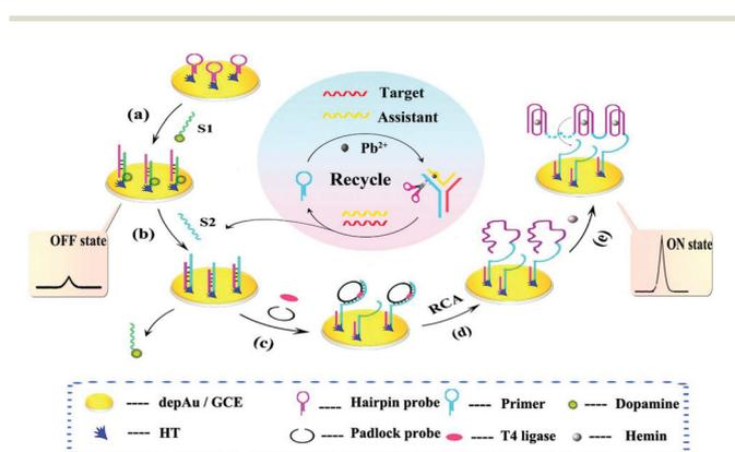
**Fig. 19** Schematic diagram of the dual amplified assay: (a) modification of S1, (b) displacement of S1 by S2, (c) incubation of T4 ligase and padlock probe, (d) RCA process, and (e) the formation of Hemin/G-quadruplex. (Reprinted with permission from ref. 87. Copyright 2015, American Chemical Society.)
