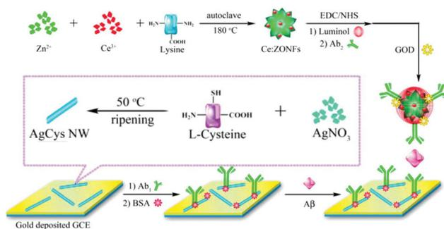
**Fig. 14** Schematic illustration of synthesis process of Ab<sub>2</sub>-GOD@Ce:ZONFs-Lum signal probe and preparation process of the AgCys Nanowires. (Reprinted with permission from ref. 75. Copyright 2016 American Chemical Society.)
