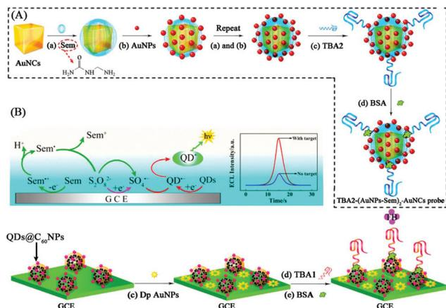
**Fig. 15** Schematic illustration of ECL aptasensor preparation process and possible luminescence mechanism: (A) fabrication of  $\text{TBA}_2$ -(AuNPs-Sem)-AuNCs signal probe; (B) fabrication of CdTe QDs@C<sub>60</sub> NPs, and (C) possible ECL mechanism of the QD-based ECL system. (Reprinted with permission from ref. 77. Copyright 2015 American Chemical Society.)
