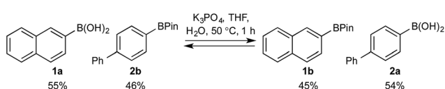
Scheme 3 Speciation equilibria of 1a and 2b in a basic biphasic medium.
