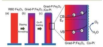
Scheme 1 Schematic illustration of the synthetic procedure of a grad-P:Fe<sub>2</sub>O<sub>3</sub>/Co-Pi photoanode. (a) Oriented Fe<sub>2</sub>O<sub>3</sub> nanobundle arrays grown on FTO substrate using RBD; (b) the prepared Fe<sub>2</sub>O<sub>3</sub> nanobundle arrays were incorporated with gradient P concentrations (the color gradient as an indicator of P content); (c) a thin Co-Pi layer was loaded on grad-P:Fe<sub>2</sub>O<sub>3</sub> photoanode
