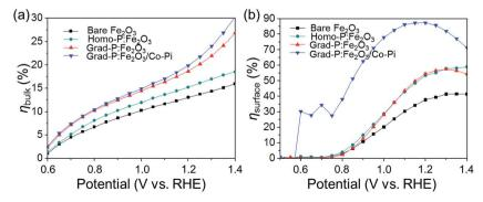
Fig. 8 Charge separation efficiency (a) in the bulk  $(\eta_{\text{bulk}})$  and (b) on the surface  $(\eta_{\text{surface}})$  of photoanodes.
