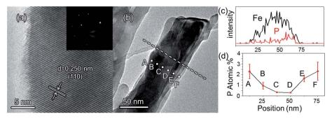
Fig. 2 (a) HRTEM image of a selected area of grad-P: $Fe_2O_3$ ; inset of (a) is the SAED pattern; (b) TEM image of a single grad-P: $Fe_2O_3$  bundle; (c) the P element distribution in a Fe<sub>2</sub>O<sub>3</sub> nanobundle (line in image b); (d) the P element concentration along the radial direction (dots in image b) (the error bar represents the standard deviation).
