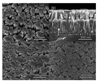
Fig. 1 SEM images of (a) top-view and (b) side-view of bare Fe<sub>2</sub>O<sub>3</sub> (500 °C for 2 h); top-view of (c) bare  $Fe_2O_3$  (750 °C for 10 min after 500  $^{\circ}$ C for 2 h) and (d) grad-P:Fe<sub>2</sub>O<sub>3</sub> (750  $^{\circ}$ C for 10 min after 500  $^{\circ}$ C for 2 h).
