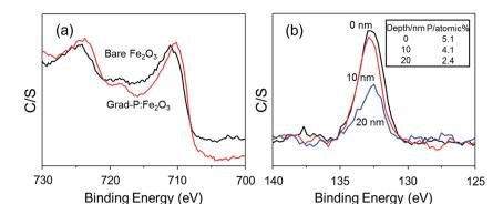
Fig. 3 (a) XPS spectra of the Fe 2p signal in bare  $Fe_2O_3$  and grad-P: $Fe_2O_3$  photoanodes; (b) XPS depth profile signal of P 2p in grad-P: $Fe_2O_3$ , where the P concentration decreases with increasing sputtering time (inset shows the P atomic concentration values at different depth).
