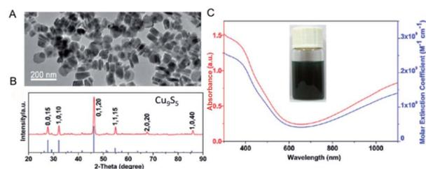
Fig. 8 TEM image (A), and XRD (B), absorption (C, red) and molar extinction coefficient (C, blue) of the prepared  $\text{Cu}_9\text{S}_5$  NPs.<sup>19</sup> Reprinted with permission from ref. 19. Copyright 2011 American Chemical Society.
