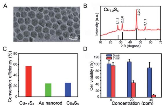
Fig. 9 (A) TEM image and (B) XRD of the obtained  $\text{Cu}_{7.2}\text{S}_4$  NPs. (C) Comparison of PTCE for  $\text{Cu}_{7.2}\text{S}_4$ , gold nanorod and  $\text{Cu}_9\text{S}_5$  under the irradiation of a 980 nm laser, respectively. (D) Cell viability after treatment with  $\text{Cu}_{7.2}\text{S}_4$  NPs at different concentration before and after the irradiation of the 980 nm laser.<sup>60</sup> Reprinted with permission from ref. 60. Copyright 2014 Royal Society of Chemistry.
