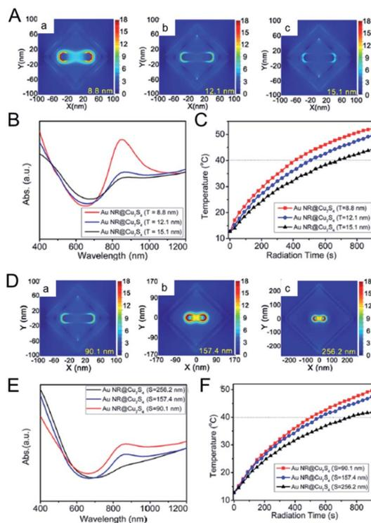
Fig. 11 Electric field distribution of Au nanorod@Cu<sub>7</sub>S<sub>4</sub> hybrid with different shell thickness ((A) a, 8.8 nm; b, 12.1 nm; c, 15.1 nm) and size ((D) a, 90.1 nm; b, 157.4 nm; c, 256.2 nm) in FDTD simulation. (B, E) The LSPRs absorption spectra and (C, F) photothermal profiles for Au nanorod@Cu<sub>7</sub>S<sub>4</sub> hybrid with different shell thickness and size.<sup>49</sup> Reprinted with permission from ref. 49. Copyright 2016 American Chemical Society.
