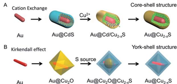
Fig. 1 Scheme of synthesizing the  $\text{Au}-\text{Cu}_{2-x}\text{S}$  hybrid based on the template method.<sup>49,63</sup> (A) Reprinted with permission from ref. 63. Copyright 2016 Wiley-VCH Verlag & Co. KGaA. (B) Reprinted with permission from ref. 49. Copyright 2016 American Chemical Society.
