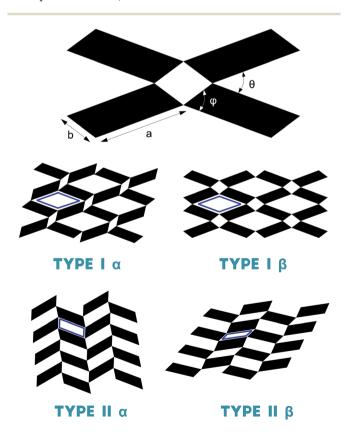
Fig. 13 Rotating rigid parallelograms systems, Type I  $\alpha$ , Type I  $\beta$ , Type II  $\alpha$  and Type II  $\beta$ . 124
