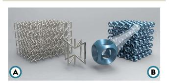
Fig. 5 (A) A typical re-entrant structure made of 3D re-entrant hexagonal unit cells and (B) a 6-hole Bucklicrystal presented by the Bertoldi group.<sup>83</sup>
