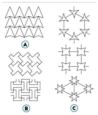
Fig. 3 Re-entrant honeycomb structures. (A) Arrowhead.<sup>66</sup> (B) Lozenge grid and square grid (from top to bottom).<sup>67</sup>(C) 3-STAR, 4-STAR and 6-STAR systems (from top to bottom).<sup>26</sup>
