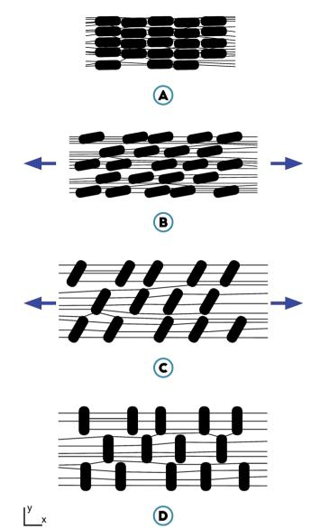
Fig. 6 Structural changes observed in microporous PTFE undergoing tensile loading in the *x*-direction.<sup>90</sup> (A) Nearly fully densified state. (B) Tension in fibrils causes particle displacement. (C) Rotation of the disc-shaped particles. (D) Fully expanded condition.<sup>89</sup>
