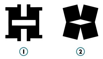
Fig. 11 Cellular plates with (1) rectangular perforations and (2) rhomboidal perforations.<sup>118</sup>
