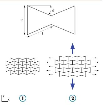
Fig. 1 Re-entrant bow-tie structure with  $\theta$  being the re-entrant angle, h/l being the cell rib length ratio and w being the thickness of the ribs. (1) In rest. (2) Tensile loading in y-direction.<sup>25</sup>
