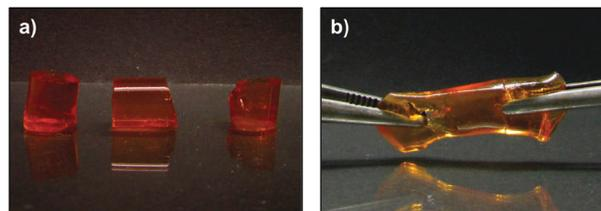
**Fig. 2** (a) Monolith OxA–GB hydrogel cut in three pieces (OxA : GB = 2 : 1 w/w). The gel was prepared using 15% w/v solutions of OxA and GB and (b) severe stretching of the monolith after reconnecting the pieces (optimal healing time = 7 days).
