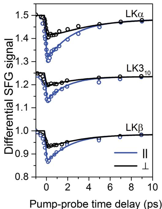
Fig. 2 Transient SFG traces of LK $\alpha$ 14, LK310, and LK $\beta$ 15 adsorbed to the air/D<sub>2</sub>O interface: experimental pump–probe transients of LK peptides adsorbed to the air/D<sub>2</sub>O interface (open circles) along with numerically simulated orientation–dependent dynamic response (solid lines). The corresponding inferred diffusion coefficients  $D_\theta$  and  $D_\phi$  are summarized in Table 1. Traces are offset for clarity.
