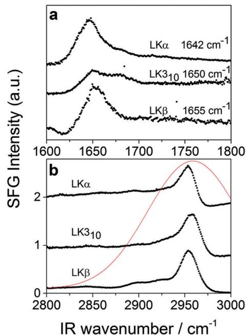
**Fig. 1** Static SFG spectra of LK $\alpha$ 14, LK $\beta$ 15, and LK $\beta$ 15 adsorbed to the air/ $\text{D}_2\text{O}$  interface (a) amide-I region using ssp polarization (see text for details) (b) using sps polarization combination in the aliphatic stretching region (see text for details). The profile of the excitation pulse is shown in red.
