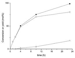
Fig. 3 Conversion of 1-octen-3-ol over Ir@CTF (squares) and evolution of products: 3-octanone (circles) and 3-octanol (triangles). The reaction was carried out at 120 °C under an inert atmosphere (N<sub>2</sub>, 2 bar) using isopropanol as solvent.
