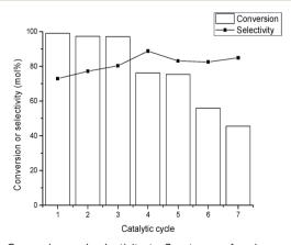
Fig. 4 Conversion and selectivity to 3-octanone for six consecutive catalytic runs. The reaction was carried out at 120 °C under an inert atmosphere  $(N_2, 2 \text{ bar})$  using isopropanol as solvent.
