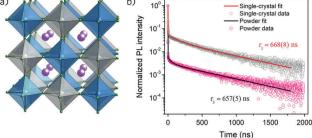
Fig. 9 (a) Crystal structure of Cs<sub>2</sub>BiAgBr<sub>6</sub>. Adapted with permission from ref. 427. Copyright 2015, American Chemical Society. (b) Time-resolved room temperature photoluminescence (PL) of single-crystal and powder Cs<sub>2</sub>BiAgBr<sub>6</sub>, including fits for the PL decay time (τ). Reprinted with permission from ref. 428. Copyright 2016, American Chemical Society
