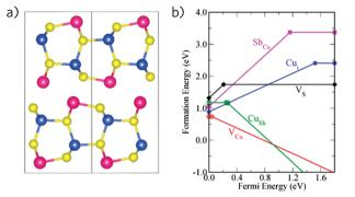
Fig. 7 (a) Crystal structure and (b) intrinsic defect formation energies of CuSbS<sub>2</sub>. Adapted with permission from ref. 253. Copyright 2014, American Chemical Society
