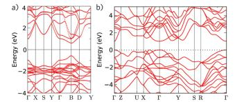
Fig. 5 Band structures of germanium-based solar absorbers: (a) CH<sub>3</sub>NH<sub>3</sub>Gel<sub>3</sub>—adapted with permission from ref. 240. Copyright 2015, American Chemical Society—and (b) GeS. Adapted with permission from ref. 241, Copyright 2013, American Physical Society.
