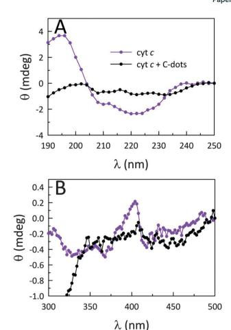
Fig. 5 (A) Far-UV CD spectra of cyt c in the presence of CA-derived C-dots; [cyt c] = 4.2  $\mu$ M and [C-dot] = 200  $\mu$ g mL<sup>-1</sup>. It is evident that the secondary structure of cyt c is completely altered by the introduction of C-dots. (B) The local heme environment of cyt c is also disturbed by the presence of C-dots, as seen in the diminished Soret band at 410 nm.
