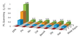
Fig. 4 Selectivity study by fluorescence emission spectrophotometry assessing impact of model analytes on emission intensity of 1 (1  $\times$  10<sup>-5</sup> M;  $\lambda_{ex}$  = 340 nm;  $\lambda_{em}$  = 609 nm; THF; 298 K). DPA: dipicolinic acid; Pic: 2-picolinic acid; Nic: nicotinic acid; Cat: catechol; BenzA: benzoic acid; Gly: glycine; Asp: L-aspartic acid.
