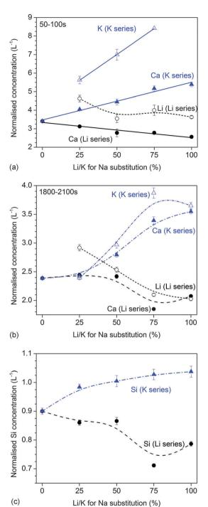
**Fig. 6** Dynamic dissolution: normalised concentrations of modifier ions at (a) the initial peak (50 to 100 s) and (b) the final stage of the experiment (1800 to 2100 s). (c) Normalised concentrations of silicon ions at the final stage of the experiment (1800 to 2100 s). Solid lines are linear regression; Li series:  $R^2 = 0.926$  (Ca); K series:  $R^2 = 0.980$  (Ca), 0.999 (K).
