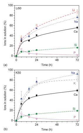
Fig. 2 Static dissolution experiments: relative ionic concentrations in Tris buffer vs. time for glasses (a) Li50 and (b) K50
