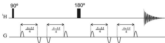
Fig. 1 A simple convection-compensated spin echo pulse sequence in which each gradient pulse has a duration  $\delta$  and a strength  $G$ , the total diffusion time is represented by  $\Delta$ , and the delay imbalance by  $\Delta\Delta$ .
