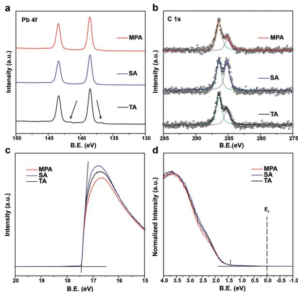
Fig. 3 (a) Pb 4f, (b) C 1s HRXPS spectra and (c) cut-off energy region, (d) valence band region of UPS spectra of MAPbI<sub>3</sub> perovskite films with various post-annealing treatments. MPA-treated films show fewer surface impurities than TA- and SA-treated films.
