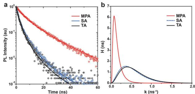
Fig. 5 (a) Time-resolved photoluminescence decay curves and (b) distributions of recombination rate constants of perovskite films with various post-annealing treatments. MPA-treated films show slower recombination rates with a narrower distribution compared to TA- and SA-treated films.
