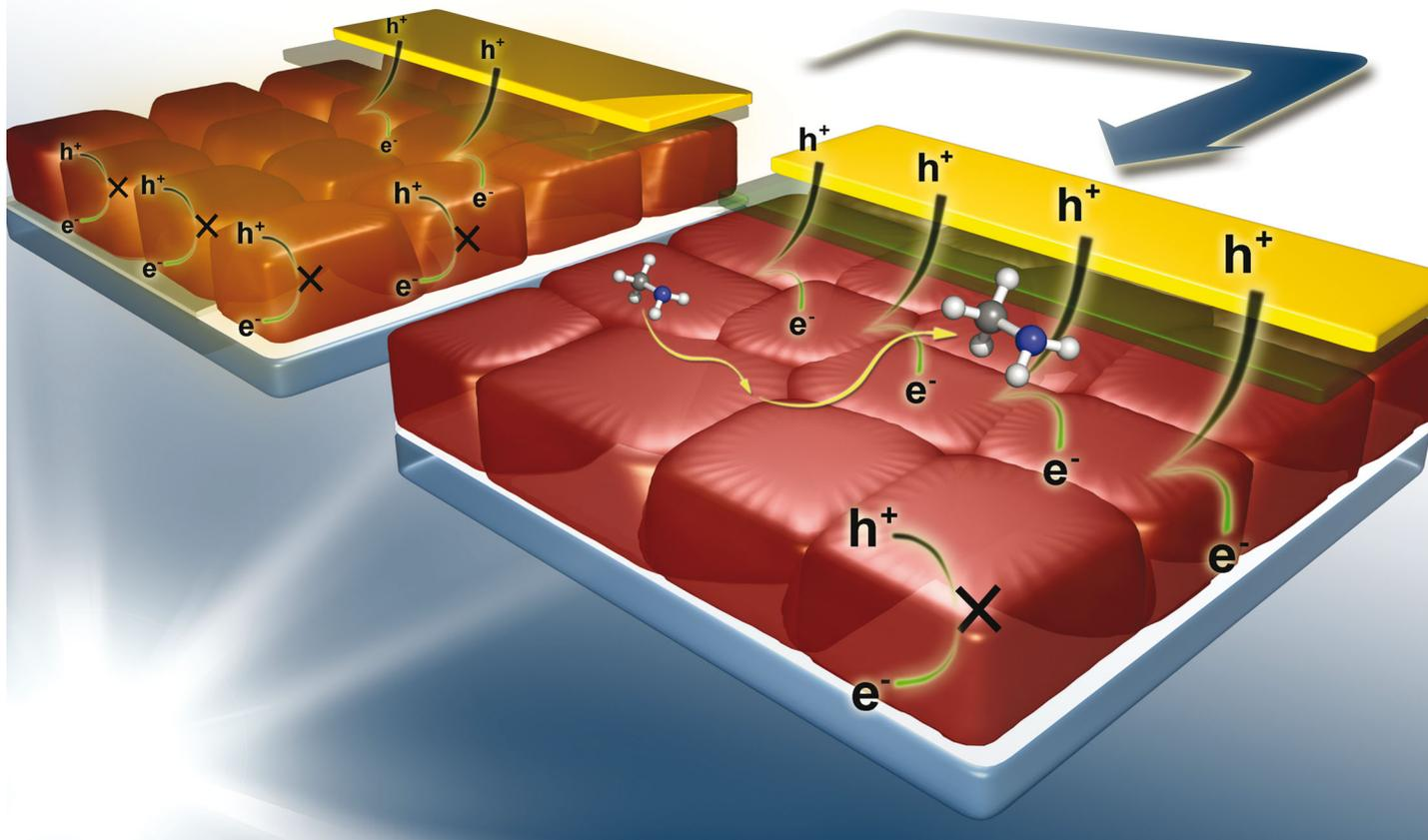
Showcasing the enhanced performance and stability of perovskite solar cells by methylamine post-annealing by Prof. Yabing Qi at the Energy Materials and Surface Sciences Unit (EMSS) in the Okinawa Institute of Science and Technology Graduate University (OIST).
