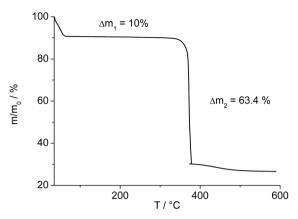
Fig. 7 Thermogravimetric curve for Al-MIL-53-ADP-lp.
