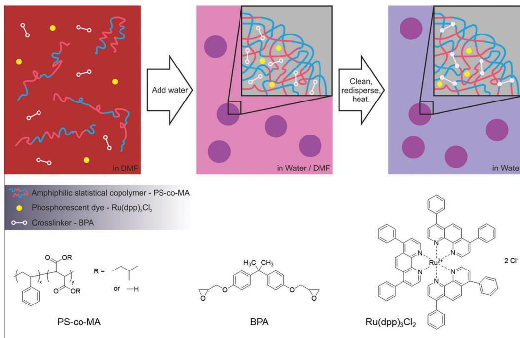
Fig. 1 Schematic illustrating the co-precipitation/crosslinking process used to prepare the phosphorescent polymer nanospheres (top), and the molecular structures of the constituent materials (bottom).
