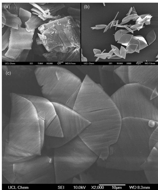
Fig. 3 Scanning electron microscopy images of (a) a sample of solvothermally synthesised MOF **1** crystals. (b and c) A sample of microwave synthesised **1M** crystals.
