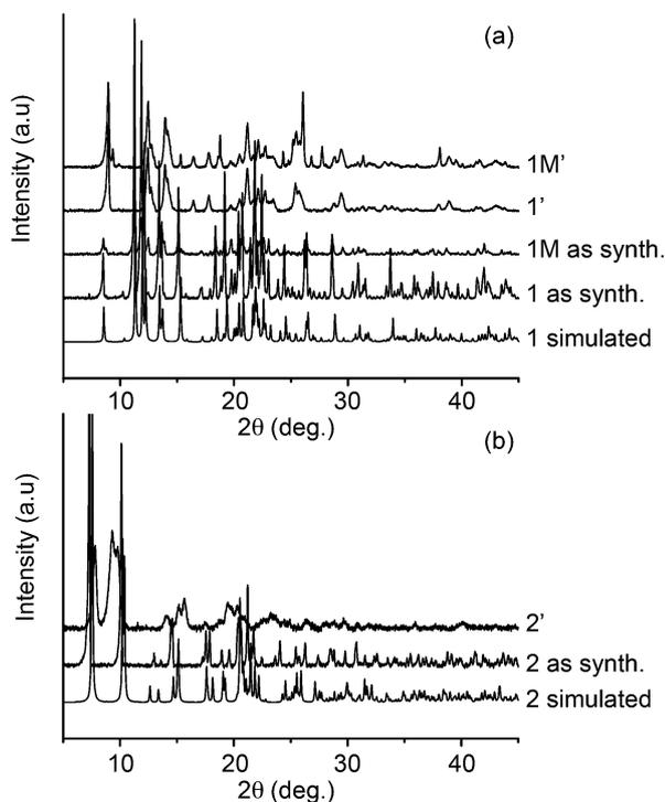
Fig. 2 (a) An overlay of powder X-ray diffraction patterns of the simulated **1** structure (as obtained from single crystal X-ray diffraction data), an as synthesised **1** bulk sample, an as synthesised bulk **1M** sample, and washed **1'** and **1M'** samples. (b) An overlay of PXRD patterns of the simulated MOF **2** structure (as obtained from single crystal X-ray diffraction data), an as synthesised bulk **2** and washed **2'** samples.
