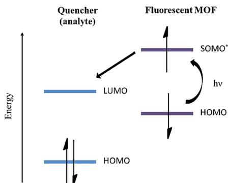
Fig. 4 Energy diagram representing the photo-induced electron transfer mechanism between MOFs in their excited state and explosive materials in the ground state (quencher).<sup>15</sup>
