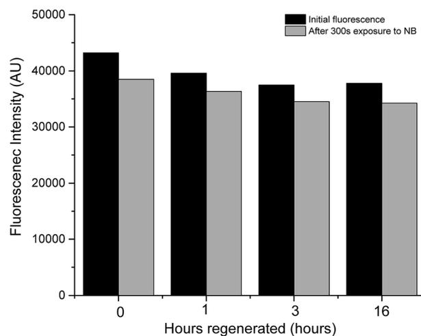
Fig. 8 Regeneration study conducted on **1'**. The graph shows the initial sensing of NB with **1'** and three cycles of sensing using the same sample towards the same analyte after 1, 3 and 16 hours regeneration at room temperature. At each time point the black bar indicates the initial fluorescence, and the grey bar the fluorescence after 300 s exposure to NB.
