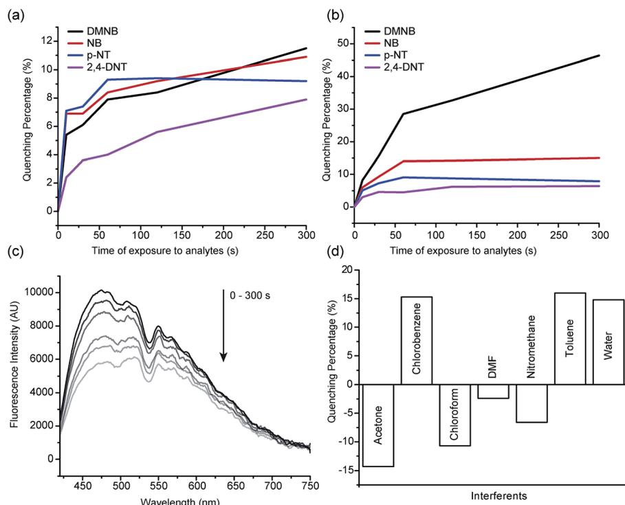
Fig. 5 (a) Fluorescence percentage quenching graphs for **1'** upon exposure to DMNB, NB, *p*-NT and 2,4-DNT. (b) Fluorescence percentage quenching graphs for **1M'** upon exposure to the same analytes. (c) Fluorescence emission profile for **1M'** upon exposure to DMNB for 0, 10 s, 30 s, 60 s, 120 s and 300 s. (d) Interference quenching percentages upon exposure to **1'** for 300 s.
