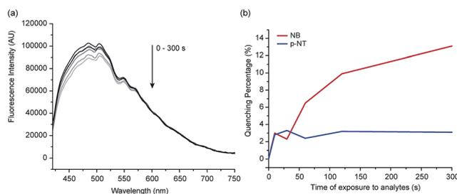
Fig. 7 (a) Fluorescence emission profile for **2'** upon exposure to nitrobenzene for 0 s, 10 s, 30 s, 60 s, 120 s, 300 s. (b) Quenching percentage plots of **2'** upon exposure to analytes NB and *p*-NT.
