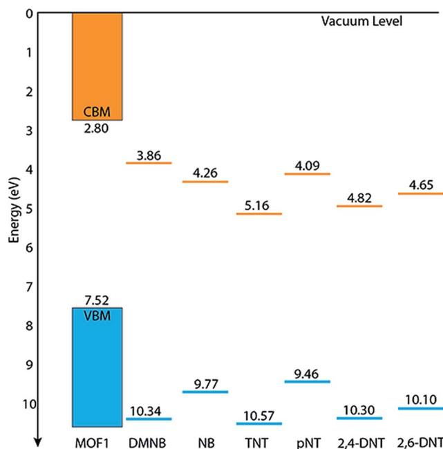
Fig. 6 Schematic of the PBE0 calculated valence band maximum (VBM) and conduction band minimum (CBM) positions for **1** and the IPs and EAs for the 6 analytes.
