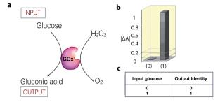
Fig. 4 (a) Schematic representation of a biocatalytic YES logic gate. (b) Bar presentation of the YES gate UV-vis absorbance outputs at  $\lambda = 500$  nm. (c) Truth table of the corresponding operation. Adapted with permission from ref. 27. Copyright (2006) American Chemical Society.
