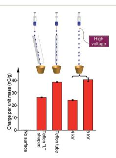
Fig. 4 An electrical potential of  $\sim$ 4–5 kV from a power supply was required to generate the amount of charge in a water droplet similar to that generated by contacting the droplet with either a L-shaped channel or a tube. When water droplets were not in contact with any solid surface, they did not contain any charge.
