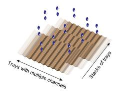
Fig. 5 Multiple L-shaped channels can be connected to form a twodimensional tray; a number of these two-dimensional trays can be stacked in the third dimension. It is proposed to install this structure in regions of abundant rainfall, or in the paths of flowing water in order to harvest the gravitational energy of water.
