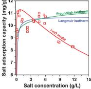
Fig. 12 Comparison of isotherm-based CDI models (Freundlich and Langmuir isotherms), and EDL models (such as the modified Donnan model). Prediction of salt adsorption capacity vs. salt concentration for two isotherm models and according to the mD model
