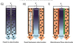
Fig. 1 (A)–(D) CDI architectures using static electrodes, including: (A) flow-between electrodes, (B) flow-through electrode, (C) membrane CDI, and (D) inverted CDI. (E) and (F) show architectures which utilize static electrodes that depart from purely capacitive behavior, including (E) hybrid CDI, and (F) a desalination battery. (G)–(I) show CDI architectures with flow electrodes, including systems with (G) feed-in electrodes, (H) feed-between electrodes, and (I) membrane flow electrode CDI.
