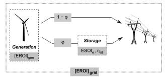
Fig. 5 A generating facility with [EROI]<sub>gen</sub> may experience curtailment, resulting in an overall EROI of [EROI]curt. Alternatively, the overgeneration may be routed through a storage facility, resulting in an overall EROI of [EROI] grid
