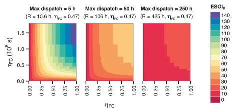
Fig. 4 Dependence of ESOI<sub>e</sub> ratio on  $\tau_{FC}$ ,  $\eta_{FC}$ , and R. Calculated from eqn (9)
