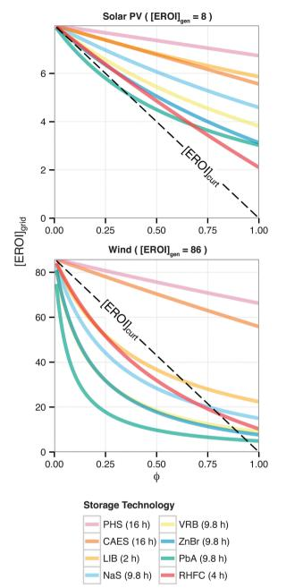
Fig. 7 Energy cost/benefit analysis of storing energy using different storage technologies. Calculated from eqn (24). Adapted from ref. 24.
