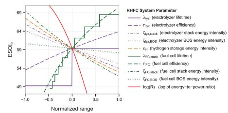
Fig. 3 Dependence of ESOI<sub>e</sub> ratio on individual system parameters. Calculated from eqn (9). The range of each parameter is specified in Table 3.
