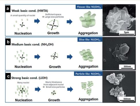
Fig. 22 Schematic diagram showing the formation process of (a) flower-, (b) slice-, and (c) particle-like Ni(OH)<sub>2</sub> under different pH conditions; corresponding SEM Images of as-prepared samples are in the Right Panel. Reproduced with permission from ref. 244. Copyright 2013 American Chemical Society
