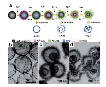
Fig. 4 (a) Schematic of synthesizing multishelled NiO hollow nanospheres using LBL self-assembly. TEM images show NiO hollow nanospheres with (a) single-shell, (b) double-shells, and (c) triple-shells. Reproduced with permission from ref. 34. Copyright 2014 Elsevier.
