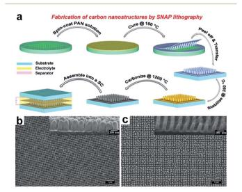
Fig. 6 (a) Fabrication of carbon nanostructures by SNAP method. (b) SEM images of top view and side view (inset) of polymer nanopillars. (c) SEM images of top view and side view (inset) of carbon nanopillars. Reproduced with permission from ref. 51. Copyright 2013 WILEY-VCH Verlag GmbH & Co. KGaA, Weinheim
