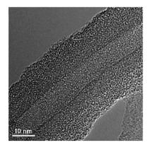
Fig. 9 High resolution TEM images of the MWCNT@PPy-MnO<sub>2</sub> coreshell structure. Reproduced with permission from ref. 92. Copyright 2009 Elsevier.
