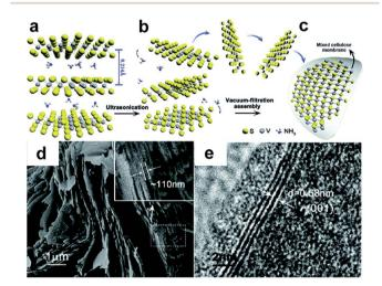
Fig. 13 VS<sub>2</sub> nanosheets for supercapacitor electrodes. S-V-S multilayers with intercalated NH3 molecules (a) is used to exfoliate thin layers of VS<sub>2</sub> (b). The transfer is accomplished by vacuum filtration and the layers are transferred on mixed cellulose membranes (c). SEM (d) and HR-TEM (e) images of the multilayer with NH3. Reproduced with permission from ref. 158. Copyright 2011 American Chemical Society.
