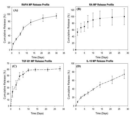
Fig. 2 In vitro release profiles of factors from phagocytosable microparticles: (A) Rapamycin, (B) Retinoic acid; and unphagocytosable microparticles: (C) TGF- $\beta$ 1 and (D) IL-10 in 2% Tween-20 PBS solution. Error bars on graphs represent standard deviation based on n=3 for each MP type.
