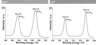
Fig. 1 (A) SEM image, (B) XRD pattern, (C) TEM image, (D) HRTEM image and XPS spectra of (E) the Bi 4f orbit and (F) the Ag 3d orbit of Ag-Bi nanoparticles. The inset of (A) shows the size distribution of Ag-Bi nanoparticles.
