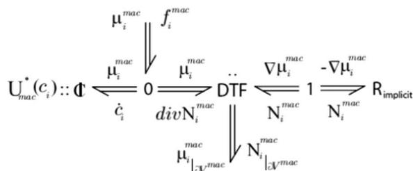
**Fig. 6** Example of an infinite dimensional bond graph model, representing the transport of a reactant across a porous media with a sink/source term connected to a microscale model (not shown here). Source: 82.
