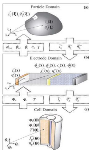
**Fig. 34** Model solution variables in each computational domain and the coupling variables exchanged between the adjacent length scales domains. Reprinted with permission from ref. 257. Copyright 2011, The Electrochemical Society.
