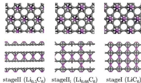
**Fig. 10** Projection views of stage II and stage I crystal structures into the grapheme planes (upper view and along the interlayer direction (lower view)). Lithium atoms are given by large circles on the top of the grapheme layers. Reprinted with permission from ref. 140. Copyright 2008, American Chemical Society.
