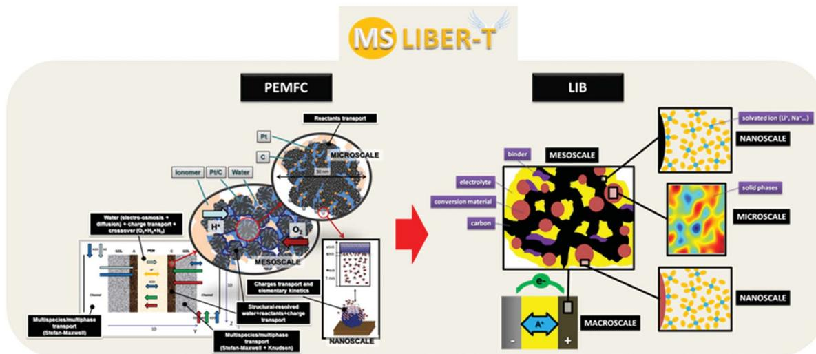
**Fig. 40** Moving from the multiscale modelling of PEMFC to the multiscale modelling of LIBs (case of conversion materials) within the framework of the computational software MS LIBER-T developed by Franco *et al.*
