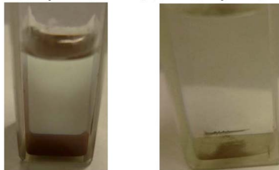
Fig. 1 Visual observation of the disproportionation of CuBr in DMSO with 0.5 equivalent (a); and 1 equivalent (b) of Me 6 -TREN after 3 h at 25 °C. Conditions: DMSO = 1.8 mL; (a) [CuBr]/[Me 6 -TREN] = 1/0.5 and (b) [CuBr]/[Me 6 -TREN] = 1/1.
