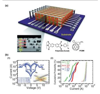
Fig. 18 (a) A schematic illustration of the three-dimensional PI memory device. The lower part shows the cross-section TEM and the chemical structures of the active materials. (b) (1) Typical I-V cures of the active layer and (2) cumulative probability data for all operative cells (160 operative cells out of 192 fabricated cells). Reproduced with permission. 19 Copyright 2010, Wiley.
