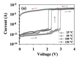
Fig. 15 /-V curves measured for the ITO/6F-HTPA PI/Al device at various temperatures under a nitrogen atmosphere. Reprinted with permission from ref. 15. Copyright 2009, American Chemical Society.
