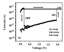
Fig. 16 I-V curves of 6F-HAB-CBZ PI. The current compliance of the first and second sweeps were set to 0.01 A, while the third sweep was set to 0.1 A. Reproduced with permission.7 Copyright 2008, Wiley
