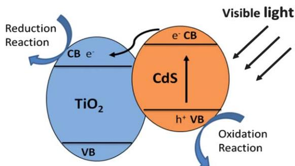
Fig. 9 Schematic illustration of charge transfer in CdS/TiO<sub>2</sub> heterostructure.
