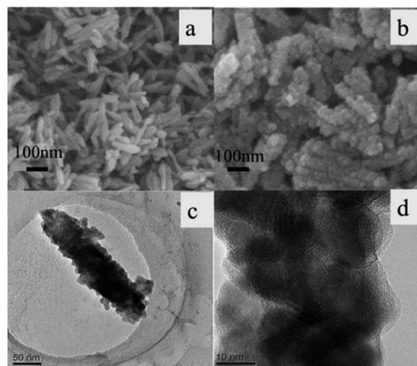
**Fig. 5** SEM images of the as-prepared TiO<sub>2</sub> nanorod film before (a) and after (b) coating with CdS nanoparticles at high magnification; TEM image of a single CdS/TiO<sub>2</sub> core/shell nanorod (c) and high-resolution TEM image of a single CdS/TiO<sub>2</sub> core/shell nanorod (d) (reprinted with permission from ref. 45, copyright 2007 Elsevier).
