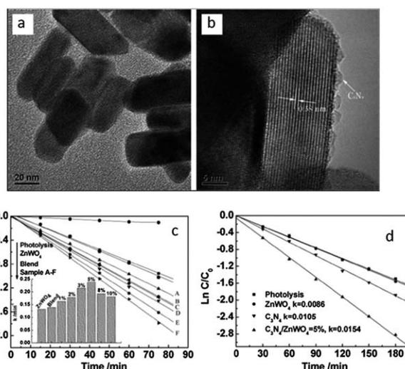
**Fig. 13** The morphology of  $ZnWO_4$  and  $C_3N_4$ /ZnWO<sub>4</sub> photocatalysts: (a)  $ZnWO_4$  (b)  $C_3N_4$ /ZnWO<sub>4</sub>; pseudo-first-order rates of MB degradation over  $ZnWO_4$  and  $C_3N_4$ /ZnWO<sub>4</sub> photocatalysts: (c) under UV light irradiation ( $\lambda = 254$  nm) (d) under visible light irradiation ( $\lambda > 420$  nm) (reprinted with permission from ref. 26, copyright 2012 Royal Society of Chemistry).
