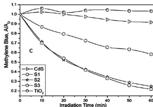
Fig. 10 (a and b) TEM and HRTEM images of CdS/TiO<sub>2</sub>; (c) the MB degradation under visible light irradiation (660 nm) in the prepared photocatalysts (reprinted with permission from ref. 24, copyright 2003 Royal Society of Chemistry).
