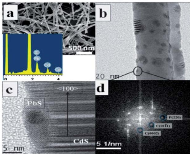
**Fig. 8** (a) SEM image of PbS/CdS synthesized by a cation exchange method, inset is EDX of the heterostructure. (b) TEM image showing a section of the nanowire with islands. (c) HRTEM indicating the presence of CdS and (d) FFT (SAED) pattern confirming the formation of PbS (reprinted with permission from ref. 69, copyright 2012 Royal Society of Chemistry).
