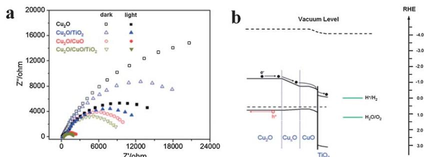
**Fig. 15** (a) EIS data of  $\text{Cu}_2\text{O}$ ,  $\text{Cu}_2\text{O}/\text{CuO}$  and  $\text{Cu}_2\text{O}/\text{CuO}/\text{TiO}_2$  nanowire array based photocathodes both in the dark and under light; (b) energy band diagram and charge transfer for  $\text{Cu}_2\text{O}/\text{CuO}/\text{TiO}_2$  (reprinted with permission from ref. 117, copyright 2013 Royal Society of Chemistry).
