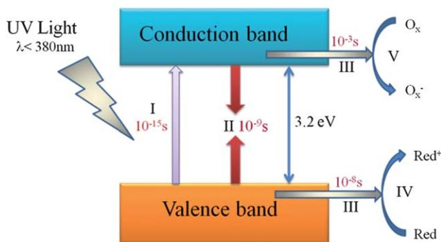
**Fig. 1** Primary steps in the photocatalytic mechanism ( $\text{TiO}_2$ ): (I) formation of electron ( $e^-$ )–hole ( $h^+$ ) pairs by photoexcitation; (II) photoinduced charge recombination; (III) photoinduced charge transportation; (IV) oxidation caused by a valence band hole; (V) reduction caused by a conduction band electron (adapted with permission from ref. 3, copyright 1995 American Chemical Society).
