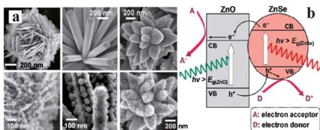
**Fig. 11** (a) SEM images of ZnO/ZnSe heterostructures; (b) schematic diagram showing the energy band structures of a ZnO/ZnSe heterostructure (reprinted with permission from ref. 90, copyright 2011 American Chemical Society).
