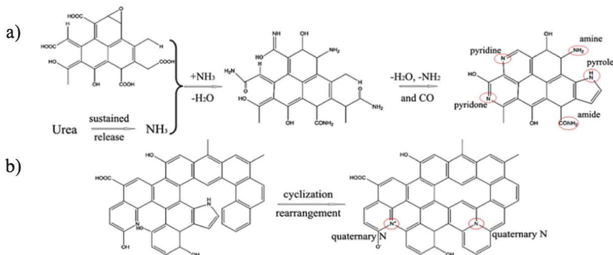
**Scheme 2** a) Nitrogen insertion routes in GO; b) Routes for the formation of a hypothetical structure of quaternary-N in GO.
