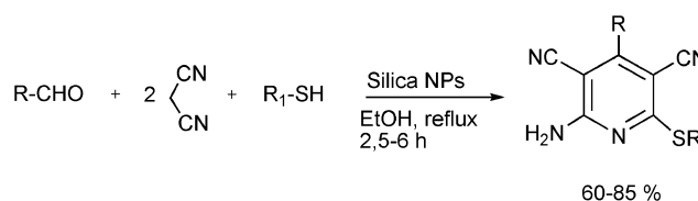
Scheme 53 One-pot three components synthesis of substituted 2-amino-3,5-dicyanopyridines.
