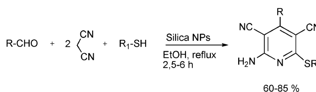
Scheme 53 One-pot three components synthesis of substituted 2-amino-3,5-dicyanopyridines.
