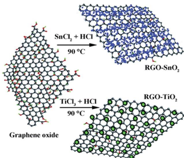
Fig. 4 One-pot synthesis of SnO<sub>2</sub>/graphene and TiO<sub>2</sub>/graphene photocatalysts. Reprinted from ref. 59.
