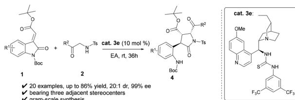
**Organocatalytic cyclization-rearrangement cascade reaction: asymmetric construction of  $\gamma$ -lactams**
