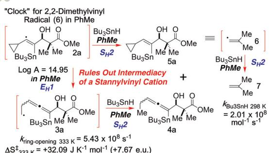
Rate constants and Arrhenius parameters for H-atom abstraction from  $\text{Bu}_3\text{SnH}$  by the 2,2-dimethylvinyl radical in PhMe. Kinetic evidence for an entirely free radical mechanism for the O-directed hydrostannation of alkynols with stannanes and  $\text{Et}_3\text{B}/\text{O}_2$
