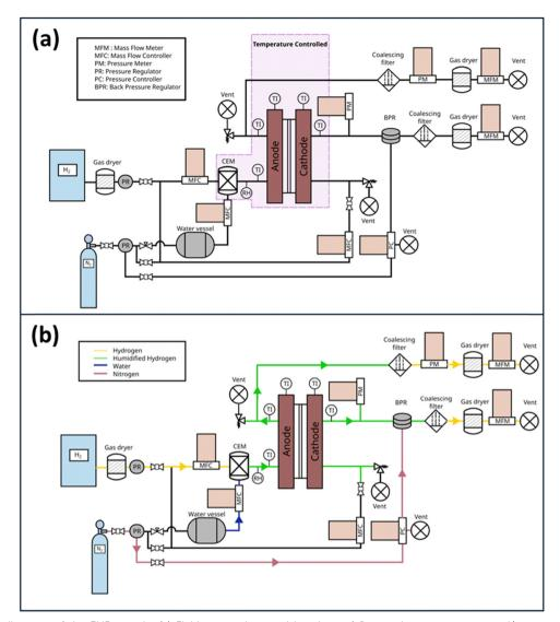
Fig. 3 Schematic diagrams of the EHP test rig. (a) Fluid connections and locations of flow and temperature control/measurement components. (b) Illustration of the fluid flow paths during standard EHP operation, showing the routing of hydrogen, nitrogen, water and humidified hydrogen streams through the system.
