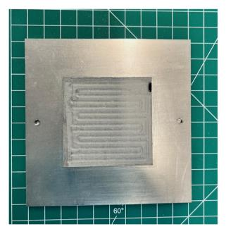
Stainless steel support that was pushed into the anode FFP, causing the membrane to puncture
