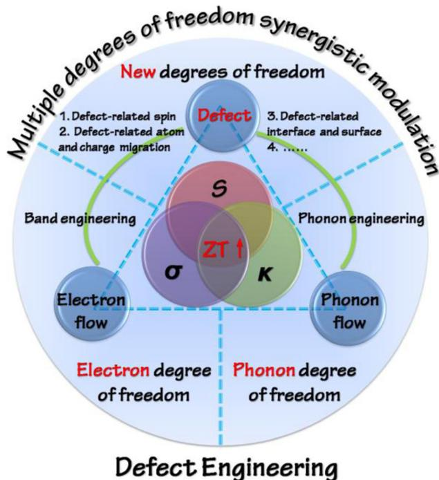
Fig. 1 Schematic representation displaying the strategies meant for optimization of  $ZT$  on the basis of defect engineering with the perception of synergistically modulating multiple degrees of freedom. Reproduced with permission from Copyright © 2016, American Chemical Society.<sup>18</sup>
