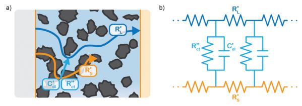
Fig. 2 (a) Schematics of the charge transfer pathways through the liquid, solid and interface of a suspension electrode, and (b) the corresponding equivalent circuit used in the TLM model. The ionic and electric conductances are described using their resistances  $R_S'$  and  $R_L'$ , respectively, while the interfacial charge transfer consists of a capacitive EDL  $\left(C_{
