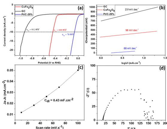
Fig. 7 (a) LSV curve of  $\text{CoFe}_2\text{O}_4$ . (b) Tafel plot of  $\text{CoFe}_2\text{O}_4$ . (c)  $C_{dl}$  plot of  $\text{CoFe}_2\text{O}_4$  obtained from the cyclic voltammetric curve at different sweep speeds. (d) Nyquist plot of  $\text{CoFe}_2\text{O}_4$ .
