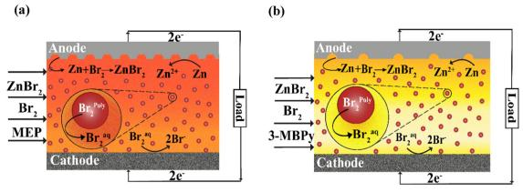
Fig. 1 Schematic of a single-flow battery with multiphase flow during discharge for the case of (a) a relatively weaker-binding BCA and (b) a strongerbinding BCA. (a) Use of a weaker-binding complexing agent, here MEP, leads to strong corrosion of the zinc anode by bromine in the continuous aqueous phase. (b) Use of strong-binding bromine complexing agent 3-MBPy, leads to reduced corrosion of the zinc anode due to lower bromine concentration in the aqueous phase.
