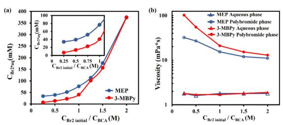
Fig. 3 Ex situ characterization of electrolytes containing initial (pre-partition) bromine concentration ranging from 0.25 M to 2 M, as well as 2 M ZnBr<sub>2</sub>, and 0.5 MEP or 3-MBPy. (a) Measured bromine concentration in the aqueous phase at equilibrium, versus initial bromine concentration. (b) Measured viscosity of each phase versus initial bromine concentration.
