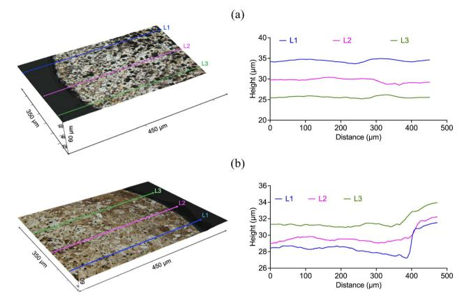
Fig. 7 Etch depth of nickel in (a) silent (60 min) and (b) after 120 s of sonication (power intensity of 300 W cm<sup>-2</sup>) with 0.1 mol dm<sup>-3</sup> of CuCl<sub>2</sub> in  $CaCl_2 \cdot 6H_2O$ :EG. In the left-hand side, the 3D reflected light images (with line profiles) are described, whereas the topographic line profiles are shown in the right-hand side of the corresponding 3D image.
