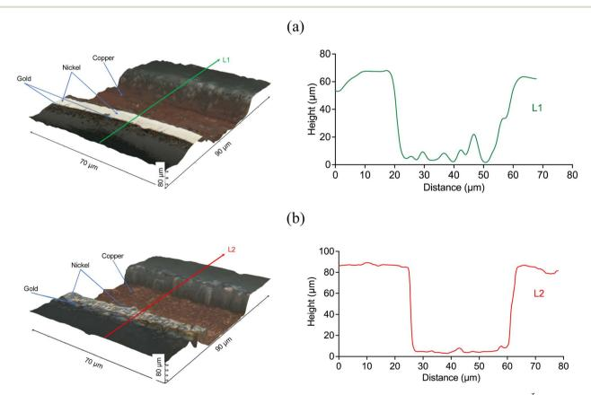
Fig. 11 3D reflected light image of the cross section of a block terminal after chemical etching (a) in silent condition (1 mol dm $^{-3}$  of CuCl<sub>2</sub> for 2 h at 50 °C) and (b) under the effect of ultrasound (0.1 mol dm<sup>-3</sup> of CuCl<sub>2</sub> and 80 W cm<sup>-2</sup>, three cycles of 10 min each).
