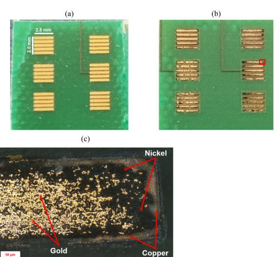
Fig. 12 (a) Initial sample of a gold-coated printed circuit board (section located at the top right in Fig. 1). (b) The same sample after 90 s of ultrasonic (200 W cm $^{-2}$ ) etching with 1 mol dm $^{-3}$  CuCl<sub>2</sub> in ChCl:2EG. (c) Reflected light image of the delimited area (red square) described in (b).
