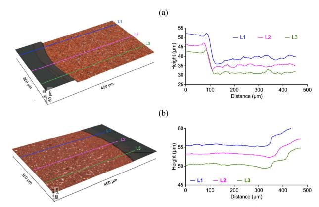
Fig. 6 Etch depth of copper in (a) silent (60 min) and (b) after 120 s of sonication (power intensity of 300 W cm $^{-2}$ ) with 0.1 mol dm $^{-3}$  of CuCl $_2$  in CaCl $_2 \cdot$  6H $_2$ O:EG. In the left-hand side, the 3D reflected light images (with line profiles) are described, whereas the topographic line profiles are shown in the right-hand side of the corresponding 3D image.
