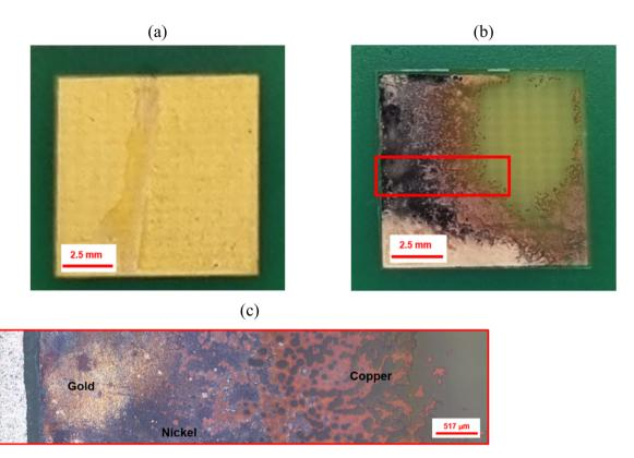
Fig. 13 (a) Single square-shape piece of a gold-coated printed circuit board. (b) The same sample after 90 s of ultrasonic (50% power) etching with 1 mol dm<sup>-3</sup> CuCl<sub>2</sub> in ChCl:2EG. (c) Reflected light image of the delimited area (red square) described in (b).
