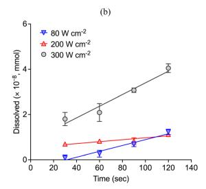
Fig. 5 Etch depth (in mmol) of (a) copper and (b) nickel under the effect of different ultrasound power intensities. Etching was carried out in  $CaCl_2 \cdot 6H_2O$ :EG with  $0.1 \text{ mol dm}^{-3} \text{ CuCl}_2$  as oxidising agent. Trend lines are also shown. Error bars represent the standard deviation from parallel experiments.
