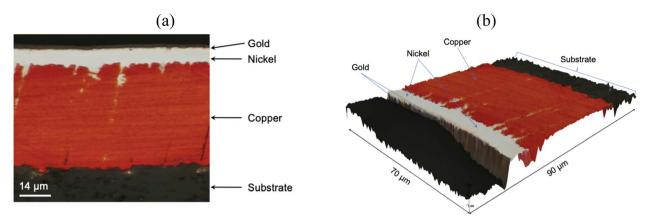
Fig. 10 (a) Cross section of a gold-coated block terminal of the PCB sample describing the distribution of gold ( $\sim$ 0.7  $\mu$ m), nickel ( $\sim$ 7  $\mu$ m) and copper ( $\sim$ 47  $\mu$ m). (b) 3D reflected light image of the cross section of the same sample.
