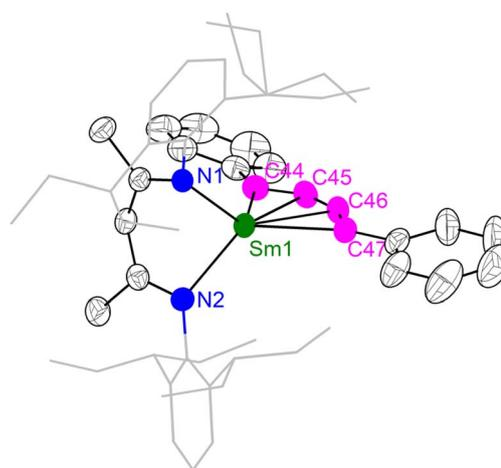
Fig. 6 X-ray crystal structure of **5-Sm** depicted as 50% probability ellipsoids. Hydrogens are omitted and the aryl substituents are shown as wireframe for clarity. Selected bond distances (Å) and angles (°): Sm1–C44 2.449(3), Sm1–C45 2.446(3), Sm1–C46 2.447(3), Sm1–C47 2.491(3), C44–C45 1.320(5), C45–C46 1.310(4), C46–C47 1.306(5), C44–C45–C46 149.0(4), C47–C46–C45 151.0(3), C44–Sm1–C47 93.0(2).
