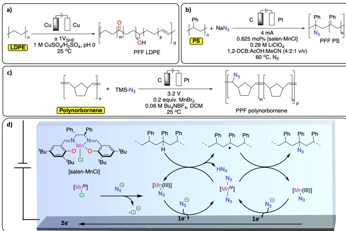
Fig. 10 Electrochemical PPF strategies for C–H bond functionalization. (a) Electrochemical oxidation of LDPE;<sup>96</sup> (b) electrochemical azidation of PS;<sup>97</sup> (c) electrochemical azidation of polynorbornene;<sup>98</sup> (d) schematic representation of the Mn-mediated oxidative azidation of PS.
