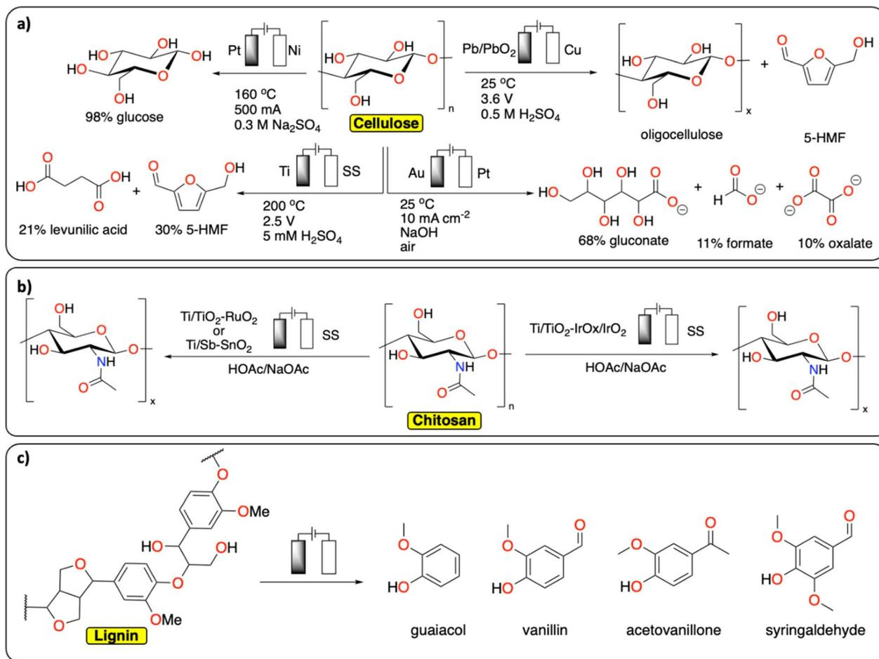
Fig. 4 Electrochemical depolymerization of biopolymers. (a) Cellulose;<sup>32–34,36</sup> (b) chitosan;<sup>39,40</sup> (c) lignin and the corresponding products obtained. For lignin, only a general scheme is provided, we refer the readers to these reviews for a more detailed description of the existing methodologies.<sup>43–49</sup>
