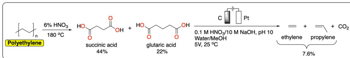
Fig. 6 Integrated tandem chemical/electrochemical depolymerization of polyethylene to ethylene and propylene.<sup>62</sup>
