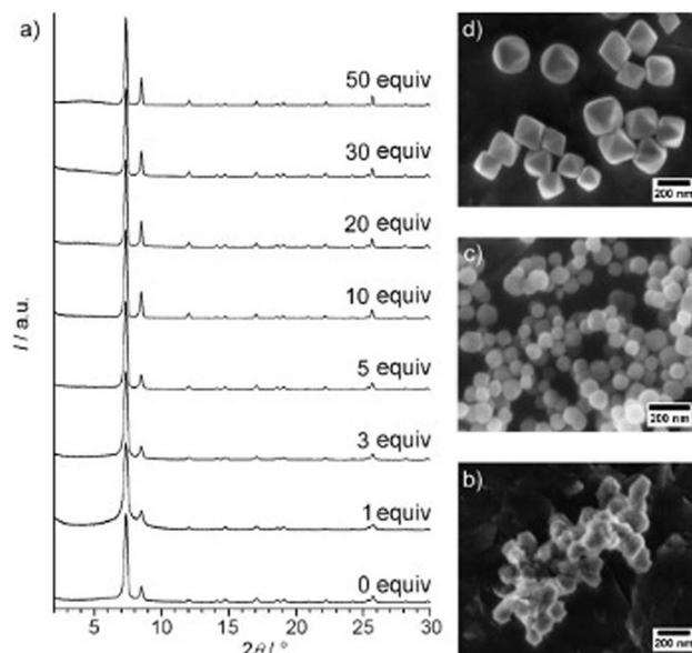
Fig. 6 (a) Powder XRD patterns of Zr-bdc MOFs prepared with different amounts of benzoic acid (given as equivalents with respect to ZrCl<sub>4</sub>) as the modulator. SEM images of Zr-bdc MOFs synthesised in the presence of (b) 0, (c) 10, and (d) 30 equivalents of benzoic acid are also given. Reproduced from Schaate *et al.* with permissions from Wiley 2011.<sup>191</sup>
