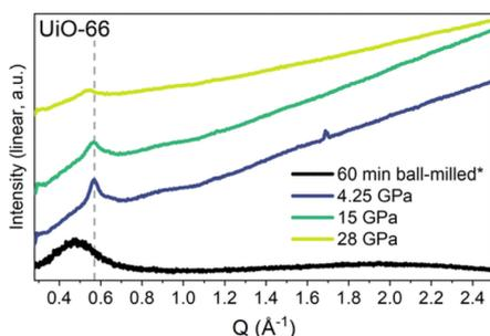
Fig. 9 PXRD data for UiO-66 after ball-milling for 60 minutes and at the maximum pressure of each *in situ* hydrostatic compression. Data were taken using either a lab source (asterisk) or a synchrotron. Data were normalised using the most intense Bragg peak (111 reflection) under ambient conditions. Figure reproduced with permission from Robertson *et al.*<sup>232</sup> Copyright 2023 American Chemical Society.
