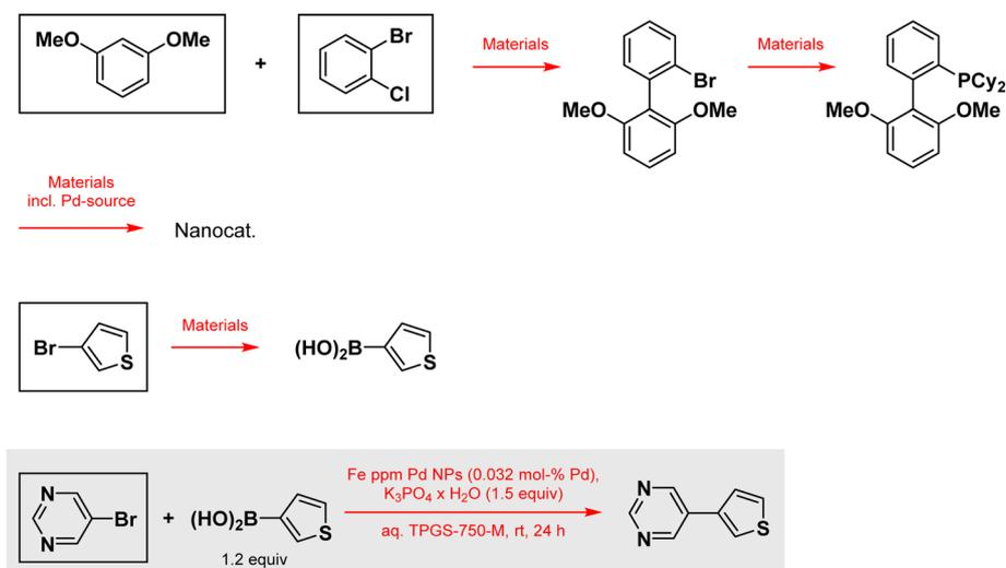
**Scheme 2** Suzuki–Miyaura coupling using ppm Pd taken from the paper in *Science* and all other reactions considered for this example. Specific data according to ref. 17 are used for framed materials. Reagents, solvents, additives and all other materials used in the outlined reactions are also considered.<sup>19</sup>
