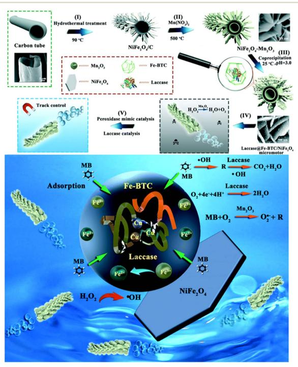
Fig. 4 Schematic representation detailing the preparation and utilization of the laccase@Fe-BTC-NiFe $_2O_4$  nanozyme hybrid micromotor. (I–V) The process begins with the synthesis of carbon tubes using kapok as a template, followed by using NiFe $_2O_4$  and laccase-immobilized Fe-MOFs to form NiFe $_2O_4$ /Mn $_2O_3$ . Finally, the degradation of organic compounds is facilitated by combined natural-enzyme and nanozyme catalysis processes. Reprinted from ref. 60. Copyright 2020, RSC.
