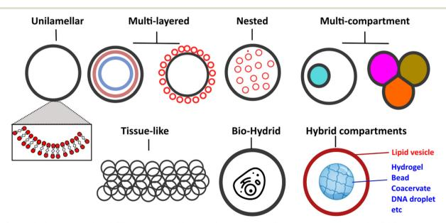
Fig. 2 Schematic showing examples of different vesicle architectures that can be controllably manufactured using microfluidic techniques.
