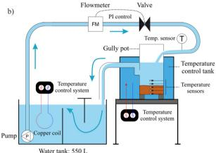
Fig. 1 (a) Image and (b) scheme of the experimental setup.
