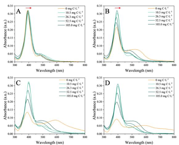
Fig. 1 UV-vis absorbance spectra of 4 mg  $L^{-1}$  nAg in the absence and presence of increasing concentration of EPS (10.5, 26.3, 52.5, 105.0 mg C  $L^{-1}$ ) at the different incubation times: (A) 2 min, (B) 2 h, (C) 24 h and (D) 72 h. SPR characteristic peak of nAg is observed at 392 nm. The red arrows in (A) and (B) represent the red shifts.
