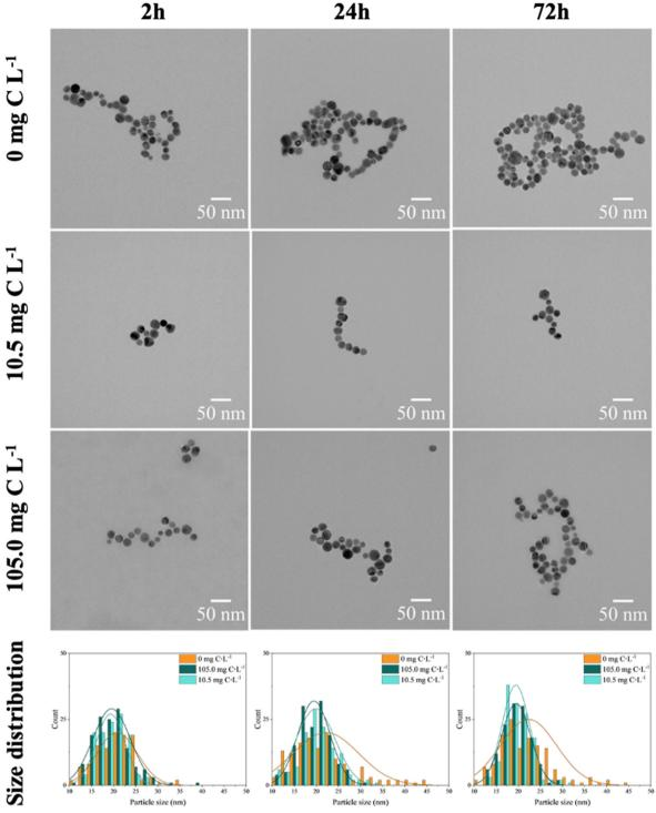
Fig. 3 TEM images of 4 mg  $L^{-1}$  nAg in the absence and presence of EPS (10.5 and 105.0 mg C  $L^{-1}$  EPS). The different size distributions were obtained counting at least 120 individual particles.
