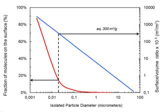
**Fig. 1** Relationship between fraction of molecules on the surface, isolated particle diameter and surface/volume ratio for spheroidal materials, adapted, with permission, from Witschger & Fabriès (2005).<sup>76</sup> Footnotes to figure: the blue line represents the correlation between isolated particles supposed to be spherical and their surface/volume ratio. The red curve represents the correlation between the diameter of these particles and the fraction of atoms at the surface.
