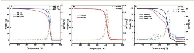
Fig. 3 TGA-DTG diagrams of three microplastics, (a) TGA-DTG of PE with different weathering times; (b) TGA-DTG of microplastic PS; (c) TGA-DTG of degradable microplastic PBAT.
