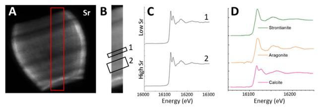
Fig. 6 Using the Sr XRF map (A), a transect (red box in (A) was selected for mapping over the Sr K-edge. (B) shows the transect in isolation and the location of region 1 (low Sr) and 2 (high Sr). The Sr K-edge XANES spectra from all pixels in each region were summed to give graphs shown in (C). XANES spectra of standards from bulk XANES measured at the beamline are shown in (D).
