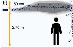
Fig. 1 Comparison of dosing O<sub>3</sub> gas, H<sub>2</sub>O<sub>2</sub>, or TEG aerosols into the office room at (a) a medium height of about 1.5 m (without the Coandă effect), and (b) at 50 cm from the ceiling (at a height of 2.5 meters) with the Coandă effect.
