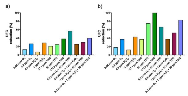
Fig. 3 Percentage of UFC reduction of (a) bacteria and (b) fungi over surfaces with triethylene glycol (TEG), ozone ( $O_3$ ) and hydrogen peroxide ( $H_2O_2$ ) nebulized individually and combined. Plots represent percentage of reduction relative to the bacteria and fungi present before the nebulization of the compounds.
